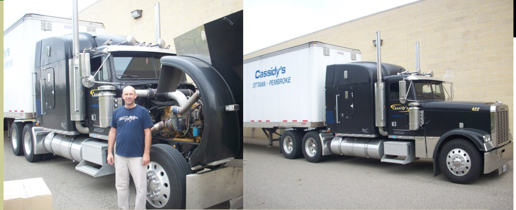
David Stufko, 1995 Freightliner truck w/ Caterpillar Model 3406E Engine with the NTF Bypass Filter system now with 2,300,000 miles as of 2012.
